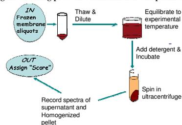
**Figure 5.** Schematic representation of solubilization protocol.
