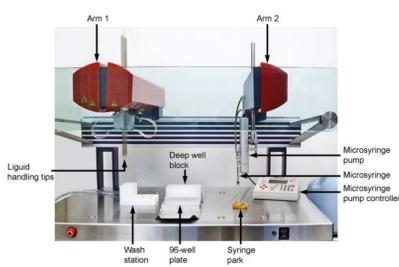
*In meso* crystallization robot (Cherezov et al, 2004)
