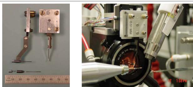
Microcollimator can hold 5 or 10  $\mu\text{m}$  aperture. Kinematic mount allows for rapid interchangeability between collimators
