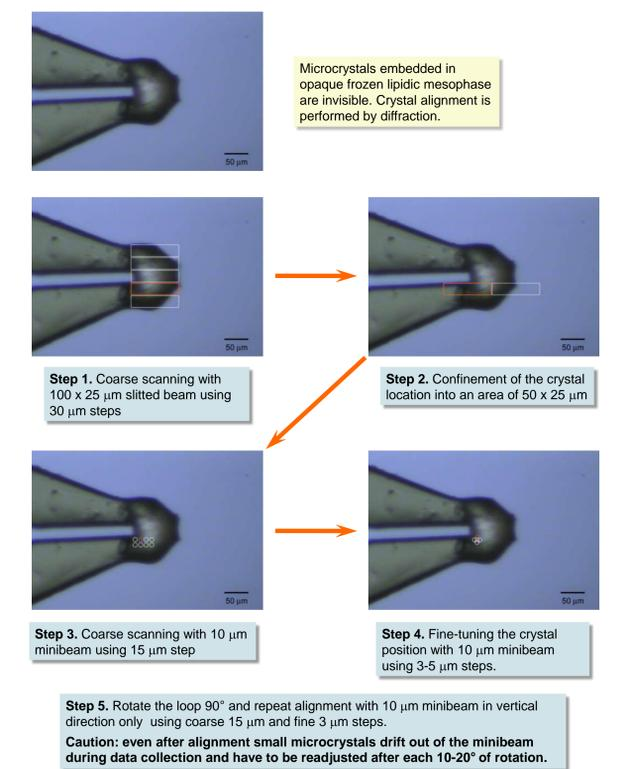
Microcrystals embedded in opaque frozen lipidic mesophase are invisible. Crystal alignment is performed by diffraction.
