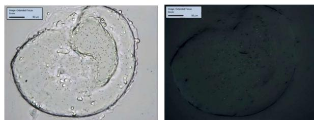
Even very small (<5  $\mu\text{m}$ ) crystals can be visually detected in most cases. Showers of small microcrystals are typical for initial hits.
