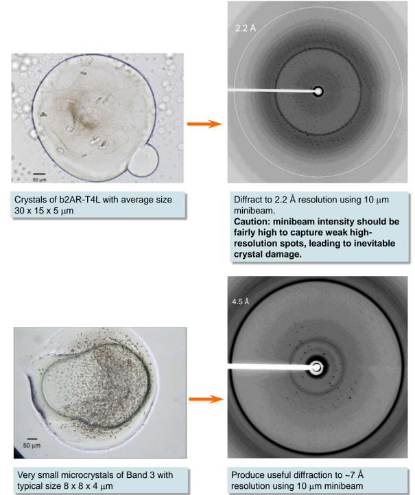
Crystals of b2AR-T4L with average size 30 x 15 x 5  $\mu\text{m}$
