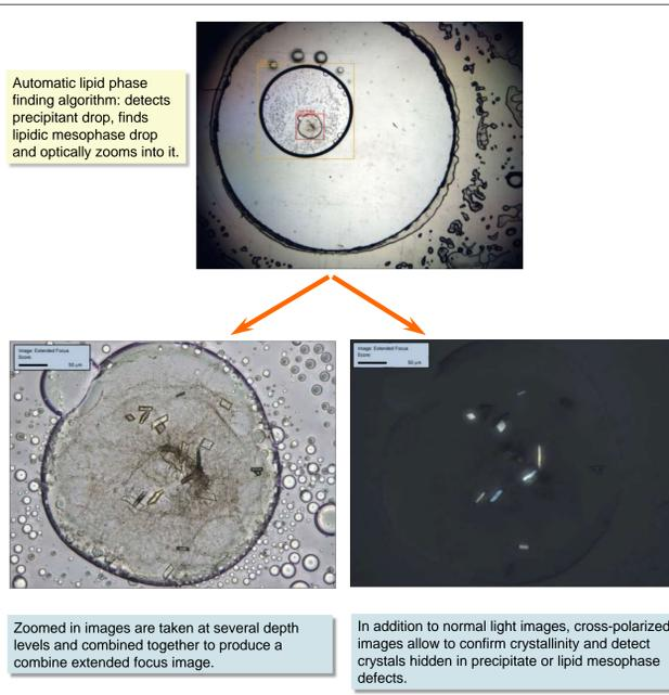
Automatic lipid phase finding algorithm: detects precipitant drop, finds lipidic mesophase drop and optically zooms into it.
