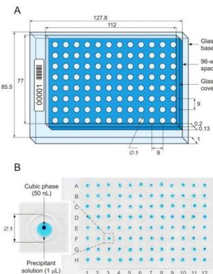
Glass sandwich plates with excellent optical properties (Cherezov et al, 2004).
